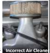
Incorrect Air Cleaner
