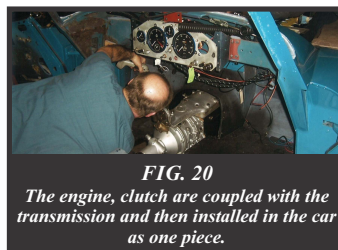
FIG. 20 The engine, clutch are coupled with the transmission and then installed in the car as one piece.
