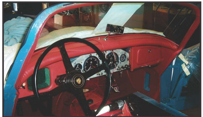
FIG. 23 The interior of the car shows the progress as the upholstery continues to go on.
